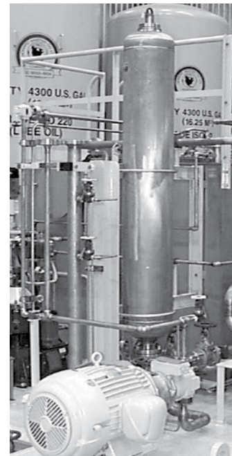
LOSAs designed for applications within turbomachinery API 614 Lube-Oil Consoles
