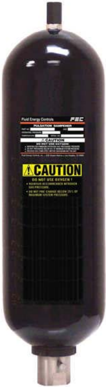
5. Smooth operator. A 5-gallon accumulator is used to dampen the pressure and volume fluctuations of the discharge from a pump. Courtesy: Fluid Energy Controls
